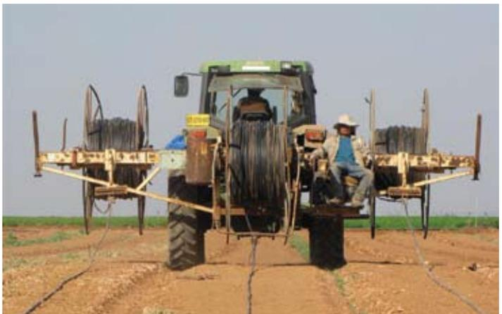
Three reels laying machine, 13000-20,000m
